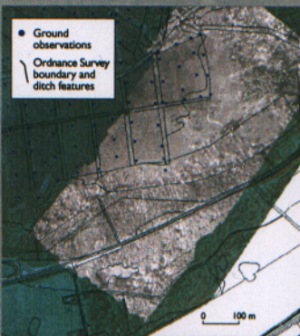
Figure 4. Orthophotograph for 1946 (panchromatic) overlaid on 1998 (colour), with OS Landline data and depth points located.
